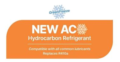
NEW AC is a high purity blend of R290 propane and R170 ethane, an ideal alternative to synthetic refrigerants R410A. GreenFreeze New AC is the natural solution for conversion of air-conditioning systems previously charged with synthetic refrigerants.
