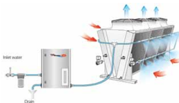
Fig. 3 Schematic for the ChillBooster™ showing how the high ambient temperature air is cooled by water droplets before passing over the coil.
